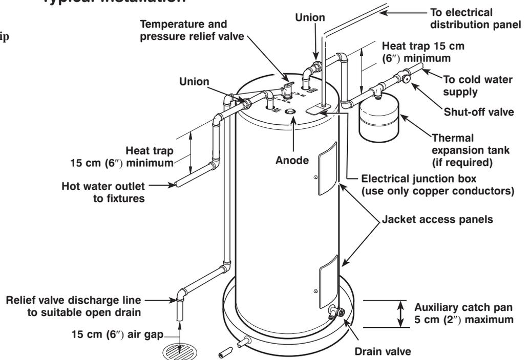
\* Some models are constructed with a side cold water inlet and will not have an opening on the top of the water heater.
