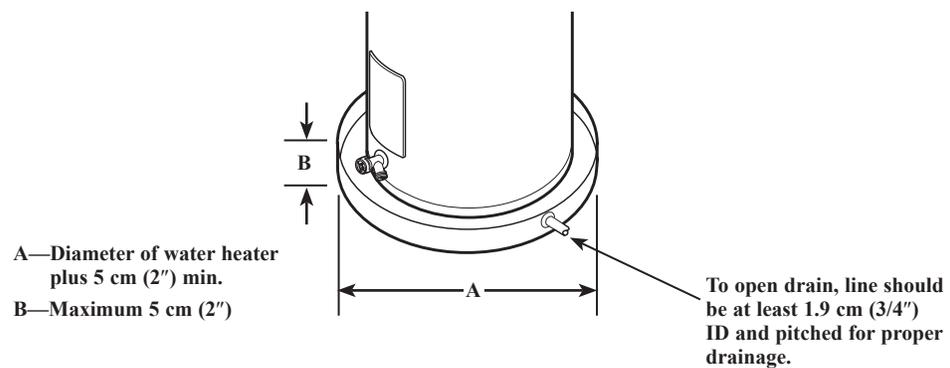
**NOTICE:** Auxiliary catch pan **MUST** conform to local codes.
